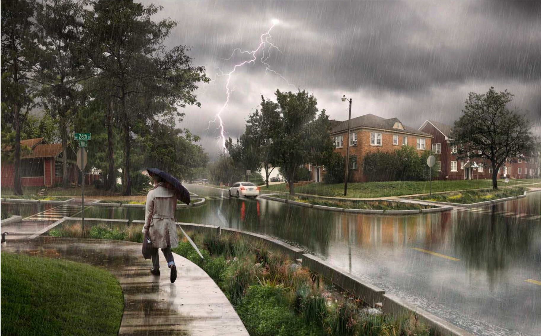
Figure 45. Rain garden bump-outs slow traffic and infiltrate stormwater. Continuous sidewalks and well-marked crosswalks improve walkability and pedestrian safety.
