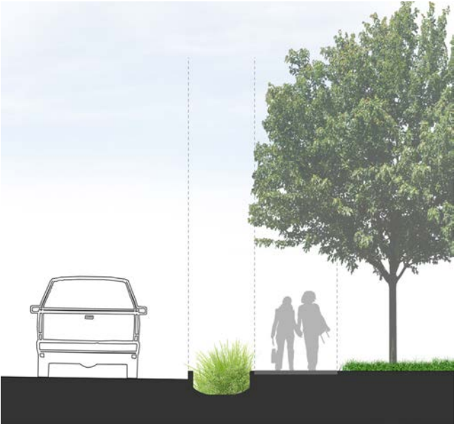
Figure 43. This section illustrates how stormwater is infiltrated in vegetated bioswales between the street and sidewalk.
