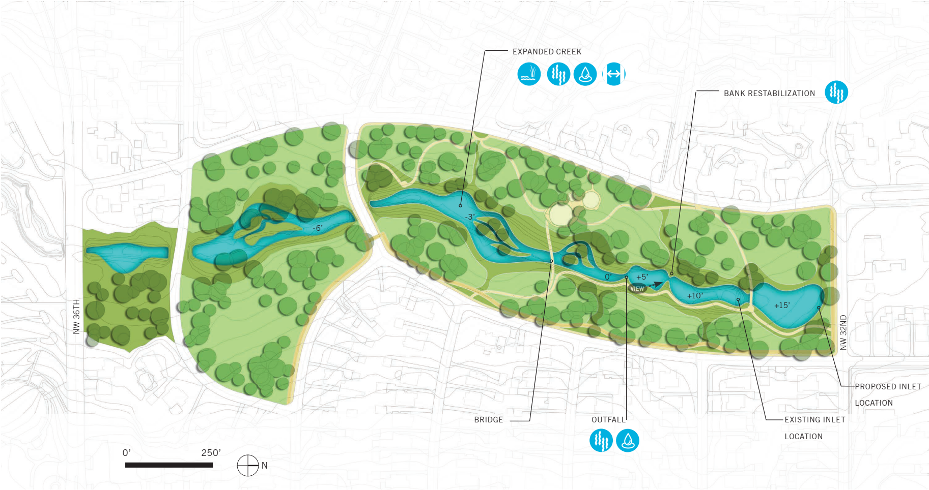
Figure 32. The design option for Guy James Creek extends and widens the creek channel to increase water holding capacity.
