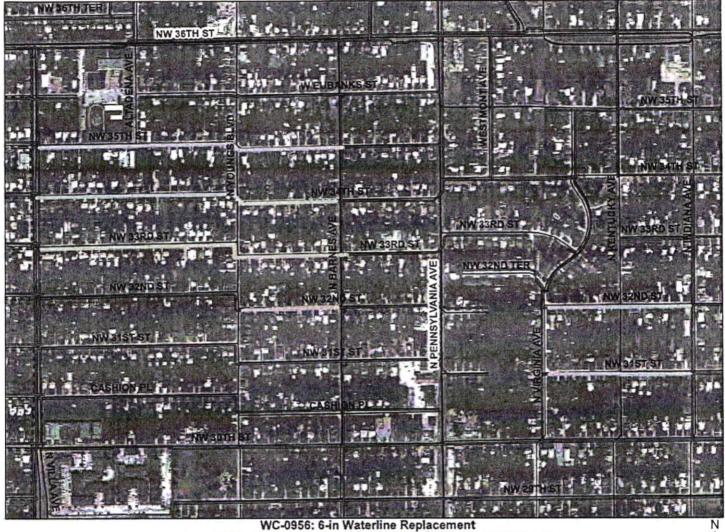
WC-0956: 6-in Waterline Replacement from N Villa Ave to N Indiana Ave b/w NW 35th St and NW 31st St 8,660 Linear feet of 6-inch Cast Iron Pipe Installed in the 1940's
