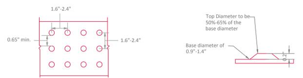
**PLAN (Enlarged) ELEVATION (Enlarged)**
