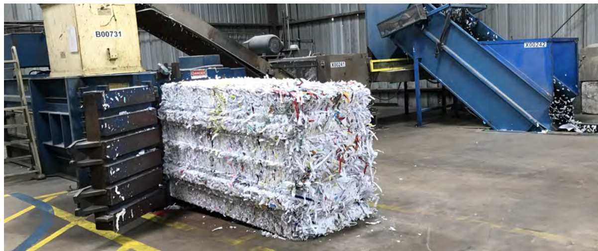
Mixed paper shredded and baled in preparation for shipment to a paper mill.
