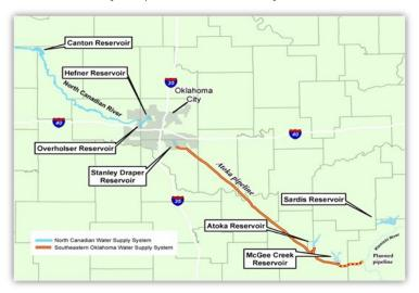
Water from the northwest travels along the North Canadian River and empties into Lake Overholser before being sent up to the Hefner Treatment Plant via a series of canals and natural tributaries. Water from the southeast travels through a 60", 100-mile pipeline that was constructed in 1962. OCWUT is currently building a second, 72" pipeline so we can continue to meet water demand for future generations.
