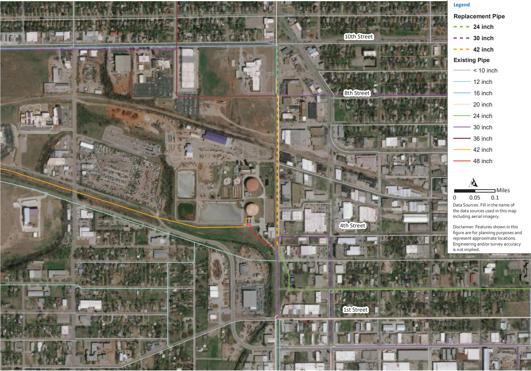
Figure 2 Proposed Replacement Pipes
