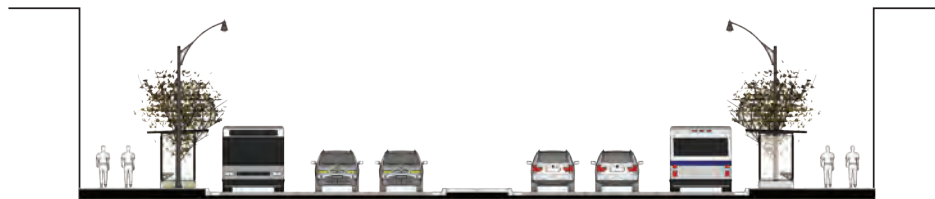
Six lane example, showing the use of Transit in the outer lanes.
