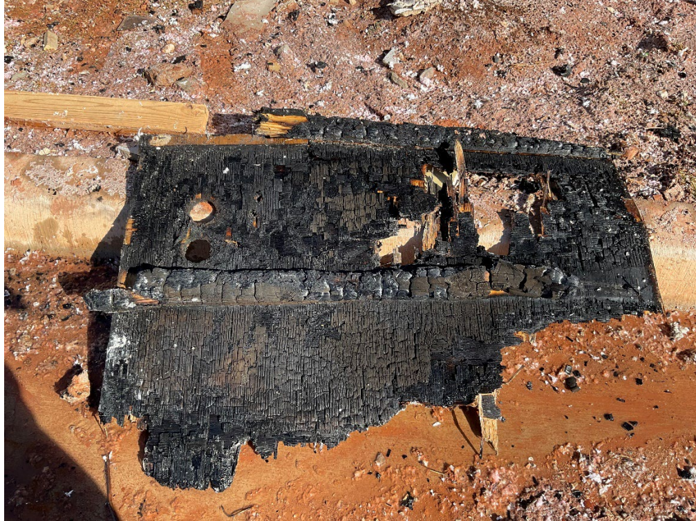
Bottom of flooring from 4 th floor electrical room; southwest area of building
