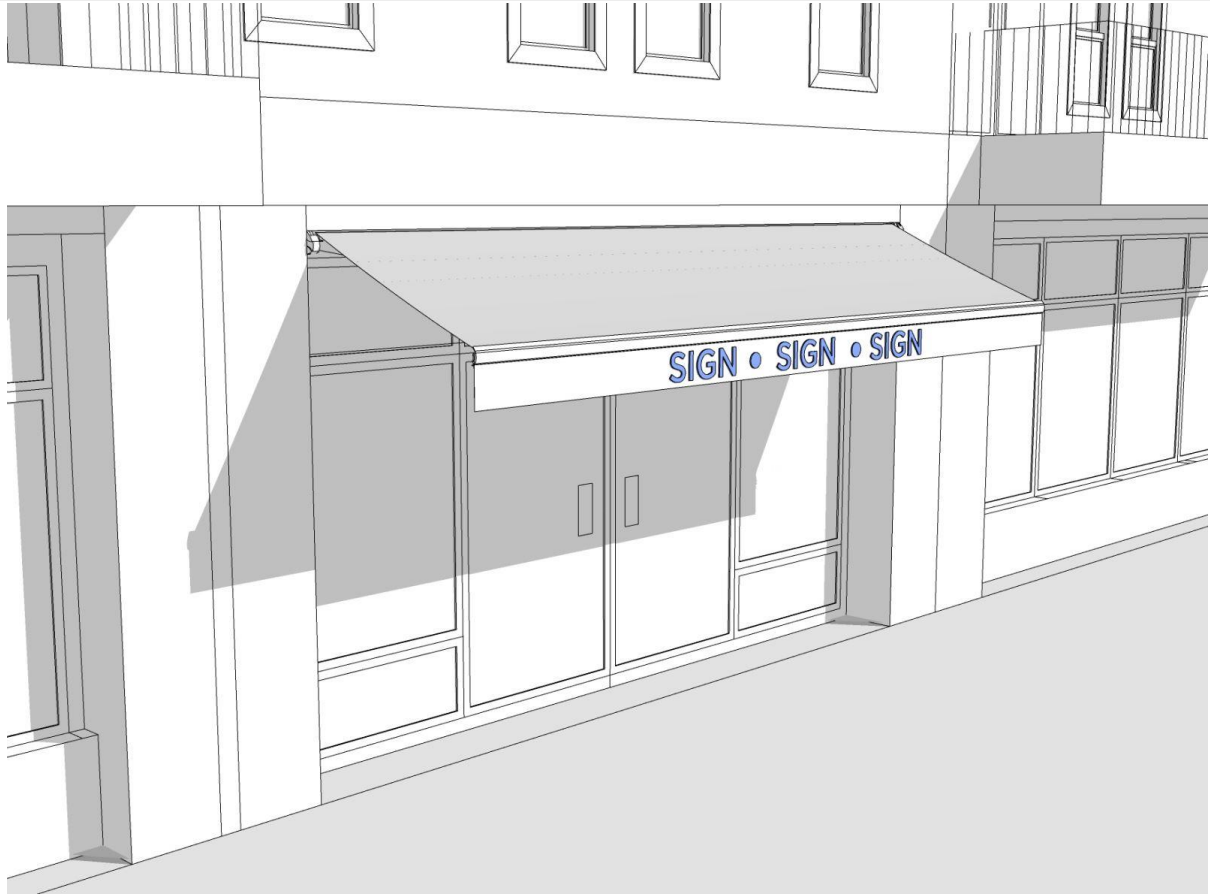
Figure 59-16108.2 Awning Signs (example)
