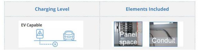
EV-READY (SPACE) is a designated parking space which is provided with a dedicated branch circuit that is not less than 40-ampere and 208/240-volt assigned for electric vehicle supply equipment in a continuous raceway or conduit terminating in a receptacle or junction box located near the proposed location of the EV parking space(s). For every two adjacent EV-Ready spaces, a single branch circuit is permitted.
