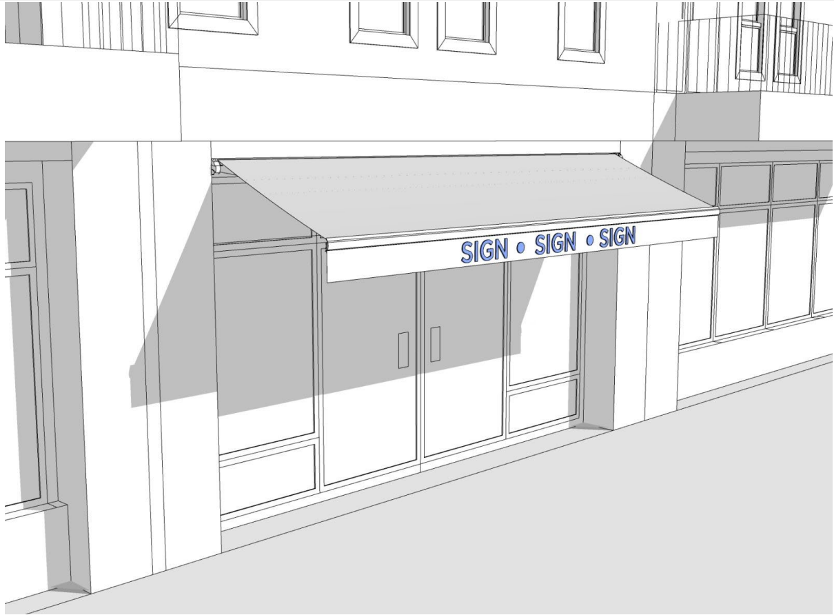
Figure 59-16108.2 Awning Signs (example)
