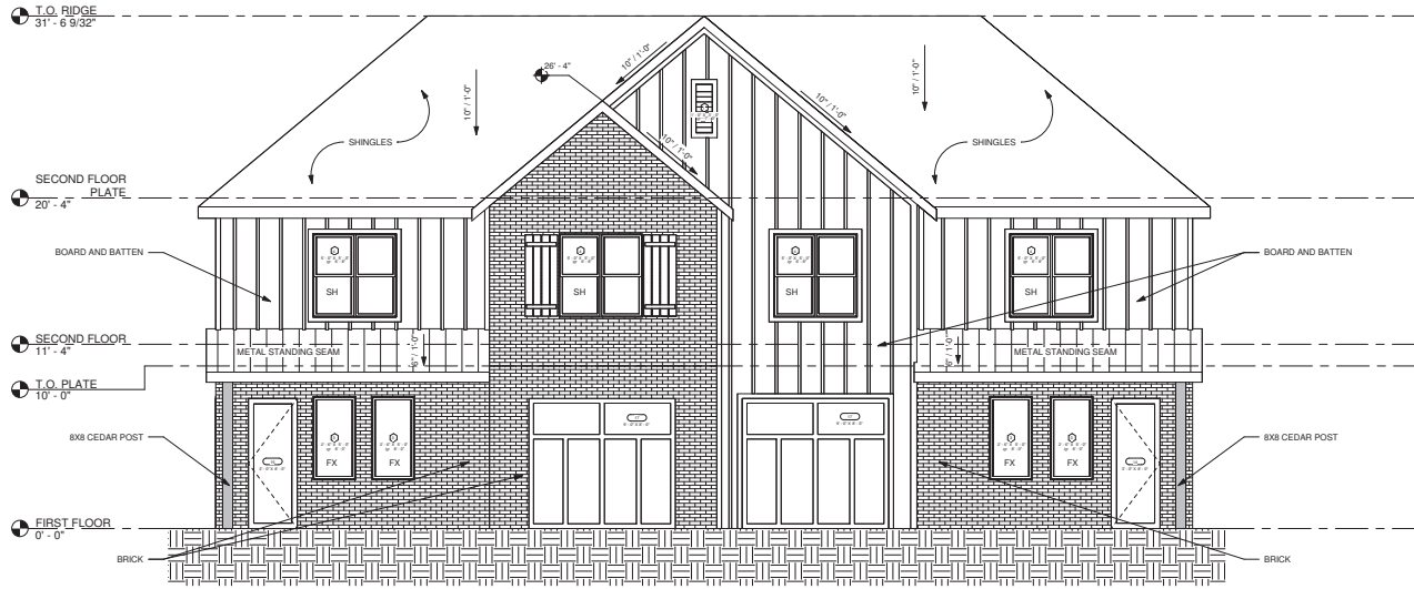
1 FRONT ELEVATION A3.0 1/4" = 1'-0"
